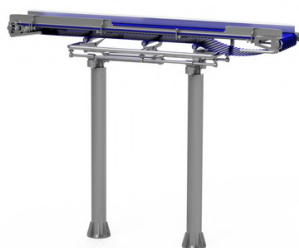
Reversible conveyer for alternate loading of two mixers
