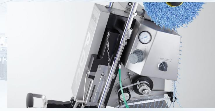
Loops can be clipped simply and securely with the automatic looper (GSE).
