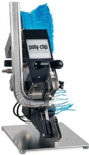
Version with pneumatic cutter and GSE (automatic looper)
